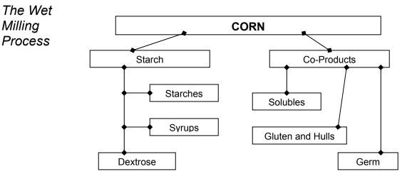
Upon arriving at a processing plant, each load of corn passes through a cleaner that removes foreign material and other impurities. Then the corn is soaked for 36 to 48 hours in hot water and sulfur dioxide. This process softens the protein (gluten) within the starch matrix while also toughening the germ.
