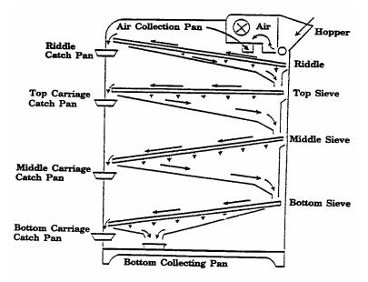
The Dockage Tester also is used to determine the percentage of broken corn and foreign material in corn. Broken corn and foreign material is a grading factor in corn.
